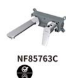
Wall-mount Basin Faucet (with pre-buried box) Finish/Color: Chrome/Black/Titanium Grey Key Parts: Φ35 Ceramic Cartridge NEOPERL Aerator Included: S.S. flexible supply tube set
